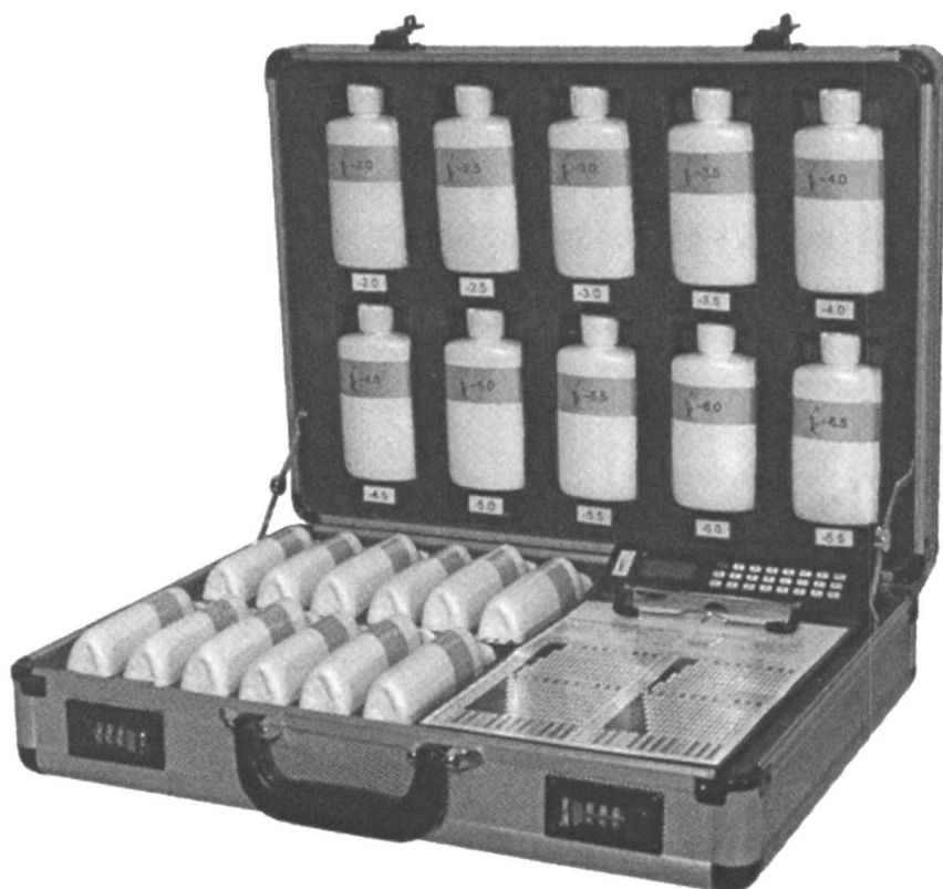
Figure 1. A modern commercially-available detection threshold test, "The Smell Threshold Test TM ." In this test, standardized forms are used with randomized presentation orders to present stimuli in a single staircase procedure. Environmental temperature is recorded, and the geometric mean of the last of four staircase procedures serves as the threshold estimate. Photograph courtesy of Sensonics, Inc., Haddon Hts., NJ USA.
